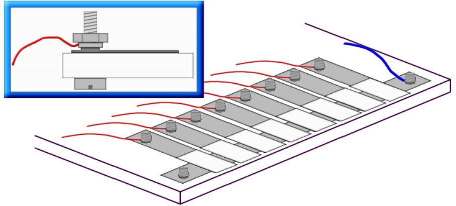
Stick the 4 feet at the bottom side of the plexyglass sheet as shown in the image.
