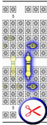
**Step 18 – Connect R7 (Resistor for the G4 Note)**
