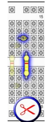
**Step 21 – Connect R10 (Resistor for the C5 Note)**
