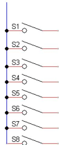
The final step is to connect each one of the switches to its resistor.
