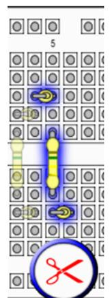
**Step 17 – Connect R6 (Resistor for the F4 Note)**
