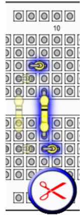
**Step 19 – Connect R8 (Resistor for the A4 Note)**
