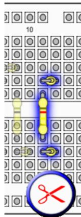
**Step 20 – Connect R9 (Resistor for the B4 Note)**
